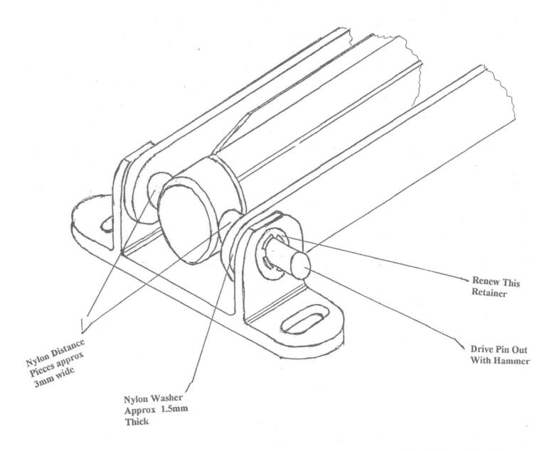
It is important to cool the power tube (in a refridgerator) for approx 20 minutes and to push the piston rod back into the tube BEFORE fitting.
